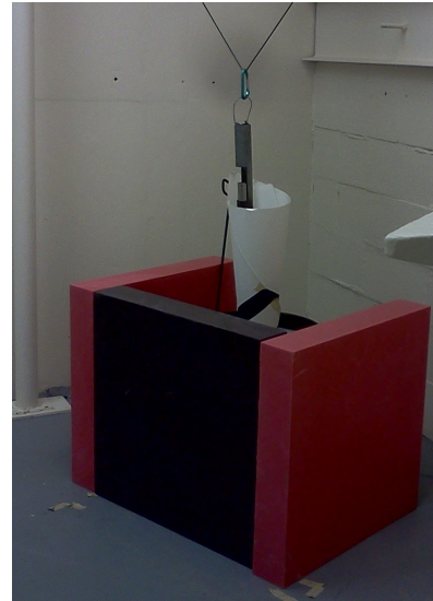
Figure 21. Picture of the source at the full height of the pulse. The funnel was made of poster board and was used to guide the source back into the container.
